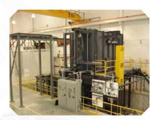
Rail systems can be mounted at grade or in a recessed pit which allows for greater visibility to operators.
