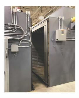
Oven is shipped with unitized sections assembled and wired to minimize installation time.
