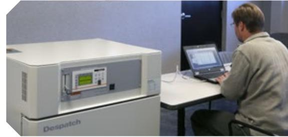
Protocol Manager™ software enables communication and control between a personal computer and up to 32 Despatch ovens equipped with Protocol 3™ or Protocol Plus controllers as well as Future Design MCT4 and MCTB controllers. The user friendly software allows oven control, recipe download and data logging.
